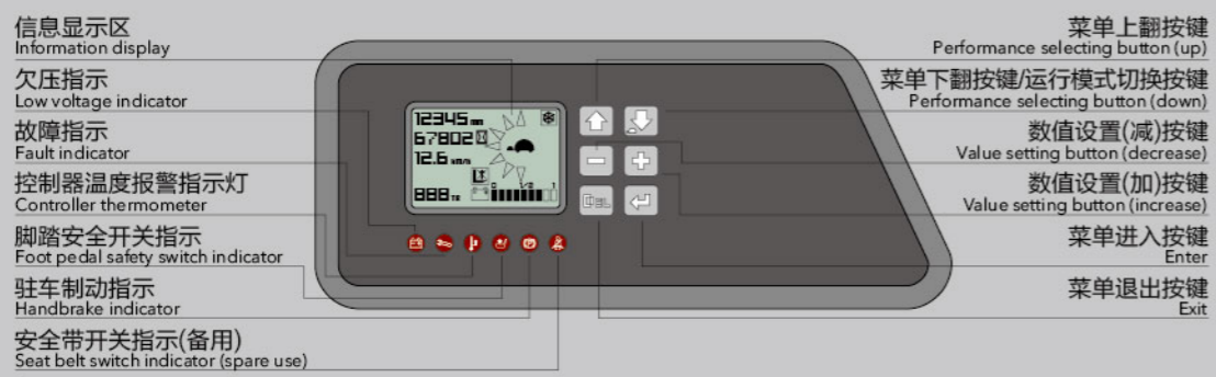
ZAPI高配仪表(用于配置号为GB2R的车型) ZAPI high level meter (for GB2R truck model)
